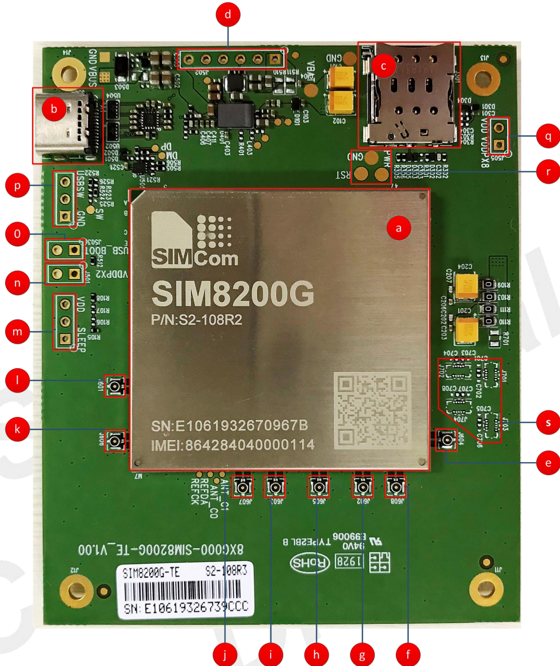
Figure 4 SIM8200G TE (front view)
